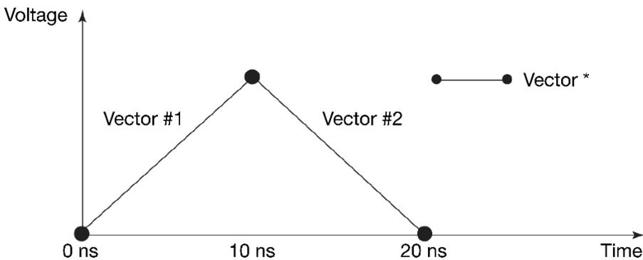
(\*) The waveform is created by specifying multiple vectors (time, voltage). Each vector can be set within the ranges of vector length and voltage.
