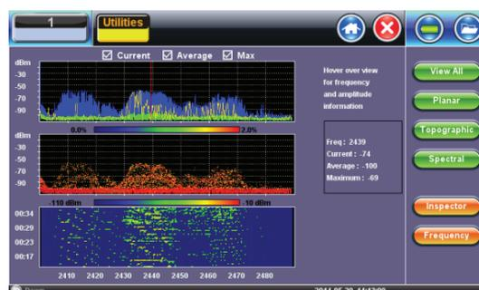
With multiple graphical format displays it helps to visualize and locate RF signals in the spectrums as well as locate and eliminate interference sources (cordless phones, microwave ovens, Bluetooth devices, etc.), discover and remedy competing access points.
