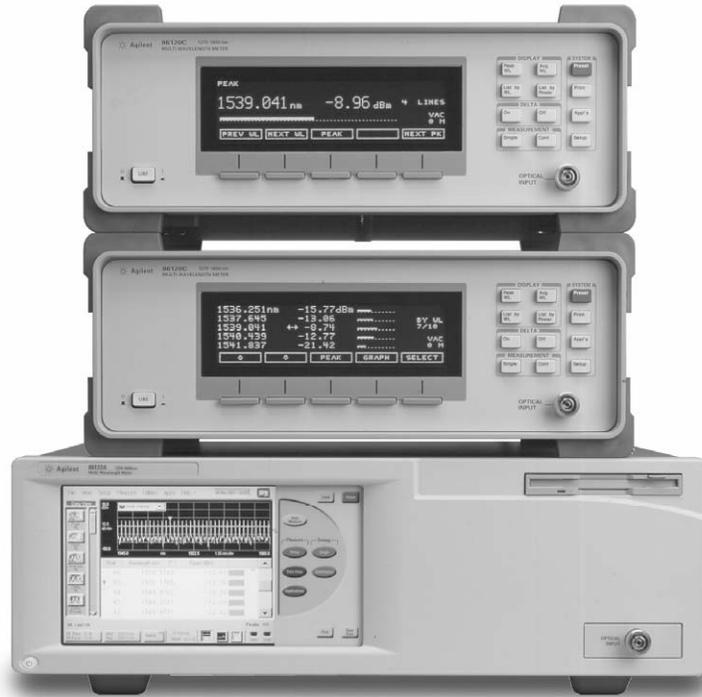
Agilent multi-wavelength meters are Michelson interferometer-based instruments that measure wavelength and optical power of laser light over a specified wavelength range. Simultaneous measurements of multiple laser lines are performed allowing measurements of DWDM signals and multiple lines of Fabry-Perot lasers. Each laser line is assumed to have a linewidth (including modulation sidebands) of less than:
