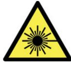
This label denotes laser output ports of instruments that contain laser sources. Refer to [Table 2](#) on page -29 for further details.
