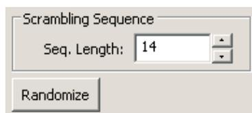
If Synchronization is set to **Auto Repeat**, the scrambling sequence is processed repeatedly without any external synchronization. The sequence will be randomized initially and will be repeated unchanged.
