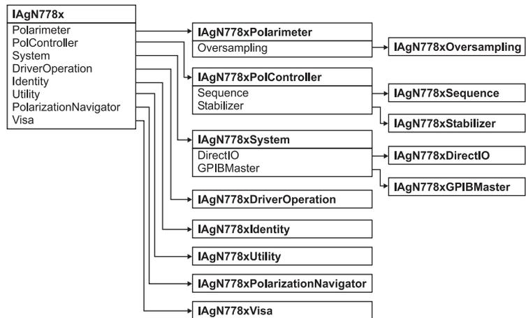
Figure 23 Diagram of COM/ActiveX-interface classes
