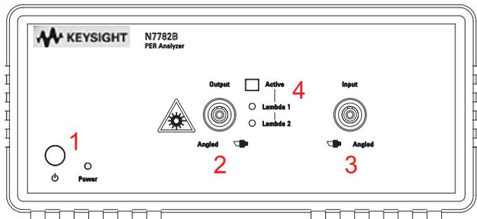
Figure 13 N7782B Front Panel with internal laser source
