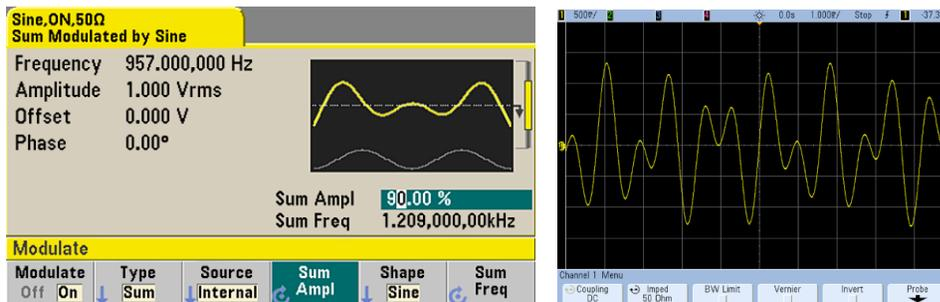
Dual-tone signal created by summing waveforms using the modulation type “Sum”.
