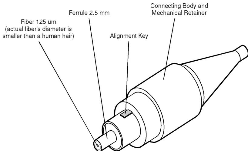
**Figure 5-1. Basic components of a connector.**
