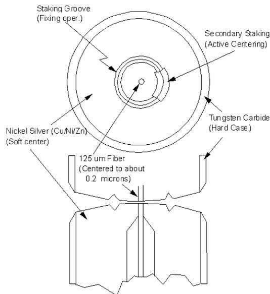
**Figure 5-3. Cross-section of the Diamond HMS-10 connector.**
