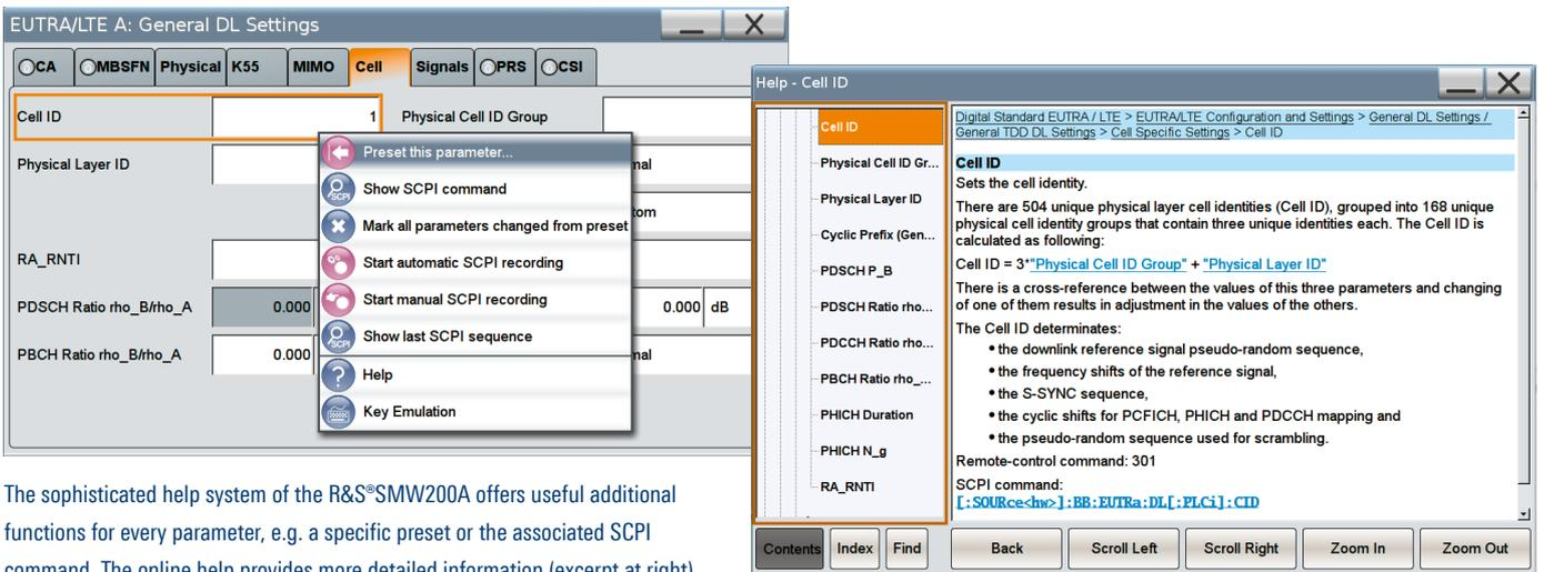
The sophisticated help system of the R&S®SMW200A offers useful additional functions for every parameter, e.g. a specific preset or the associated SCPI command. The online help provides more detailed information (excerpt at right).
