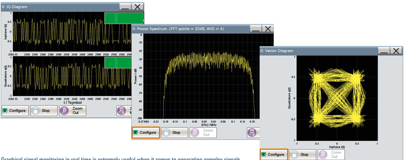
Graphical signal monitoring in real time is extremely useful when it comes to generating complex signals.
