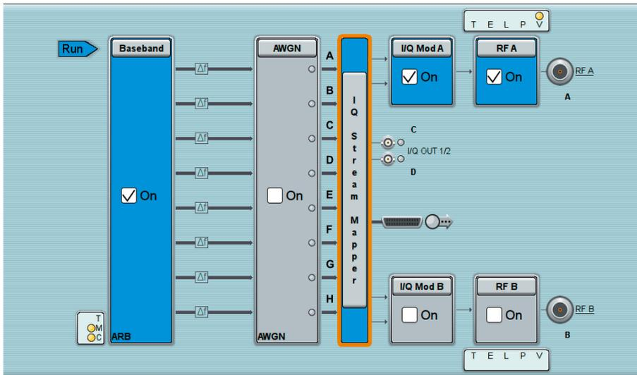
The R&S®SMW200A is the ideal generator for multi-standard radio and interference tests. In this example, it is generating eight different frequency-spaced signals that are added up in real time for receiver testing.
