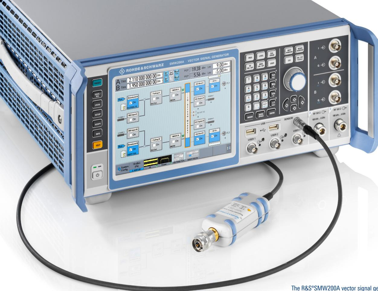
The R&S®SMW200A vector signal generator with a power sensor.
