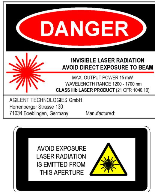
**Figure 1 USA Safety Labels (81480A, 81680A, 81640A, 81682A, 81642A, 81689A)**
