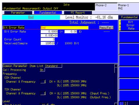
Bit Error Rate Measurement (8PSK)
